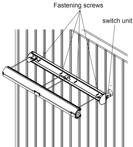
Finally, mount the cover by hanging it in the top fold of the bottom section.
