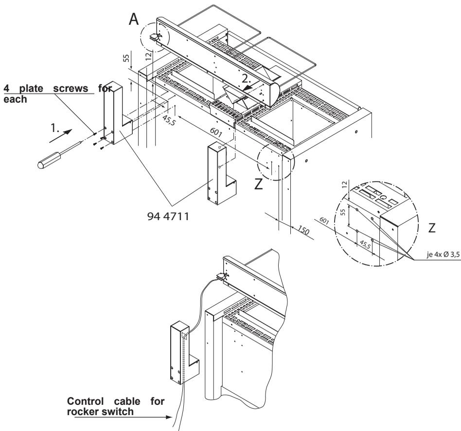
Lay the control cable for the rocker switch and heater supply with a minimum clearance of 30 mm.
