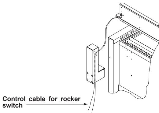
Lay the control cable for the rocker switch and heater supply with a minimum clearance of 30 mm.
