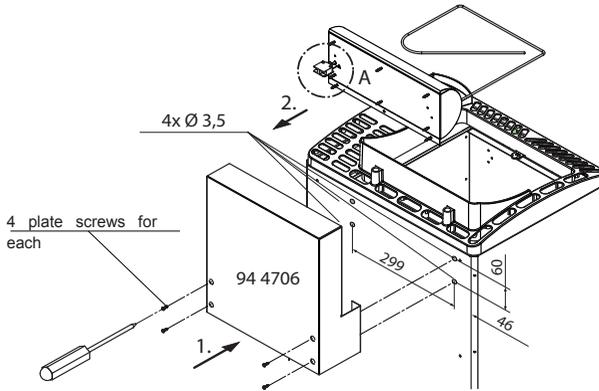
All plate screws for suspension of the heater protector.
