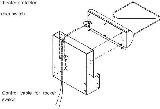
Control cable for rocker switch
