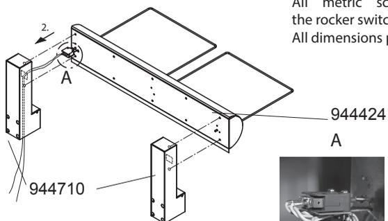
Control cable for rocker switch
