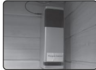
Hang up ionizer on a screw hook at the designation of oxygen ionizer
