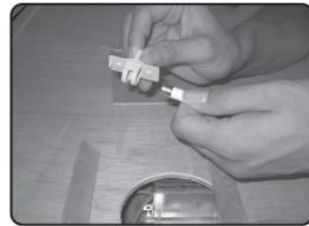
3. take fuse out, then push in a new fuse
